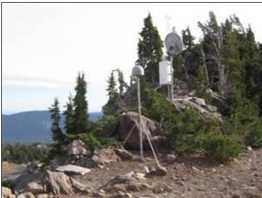
Fig. 2 Photograph showing GPS recorders installed at the Plate Boundary Observatory, Mt. Hood, Oregon, Western USA (Clement, et al. , 1999).
